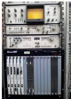
Platforma ATCA (Advanced Telecom and Computer Architecture) – Siemens/Schroff/Intel
